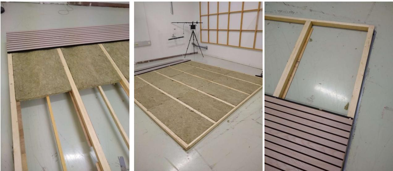
Figure A3.3. The panels were attached to the wooden frame (L3500 × W3000 × H50/200 mm). Total size of the installation was 10.5 m<sup>2</sup> (16 panels).
