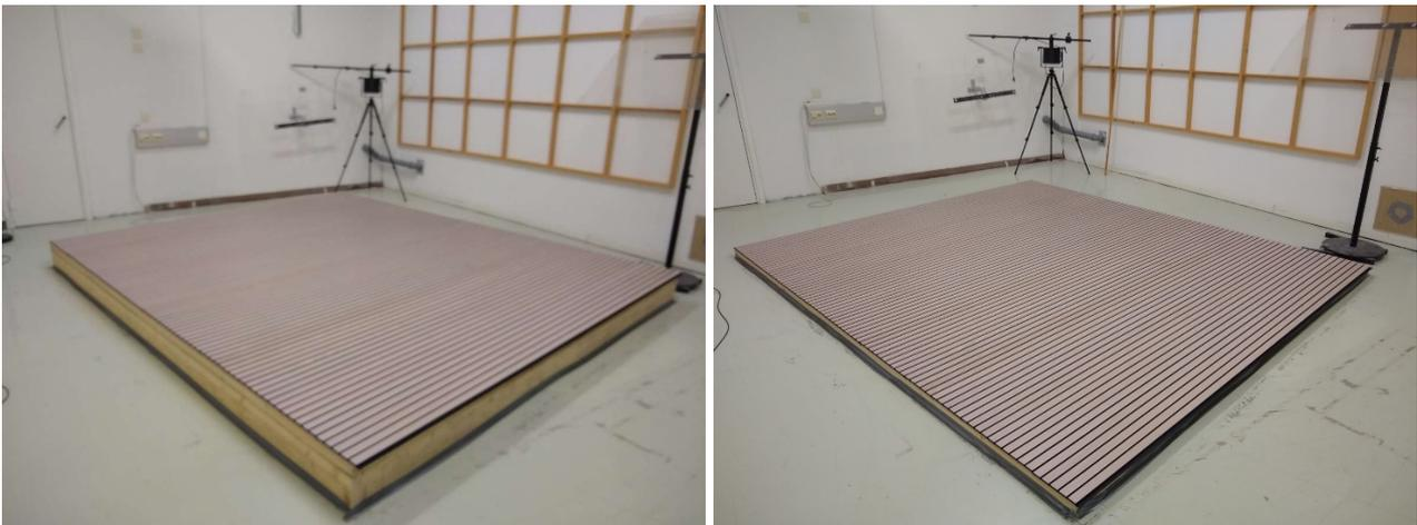
Figure A3.1. The specimens mounted on the floor of the reverberation room. Configurations 1-2 on the left and configurations 3-4 on the right.
